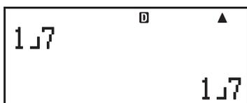
Calculator display showing  $\frac{1}{7}$  as a fraction. The screen shows  $1 \div 7$  in the top left and  $\frac{1}{7}$  in the bottom right.
